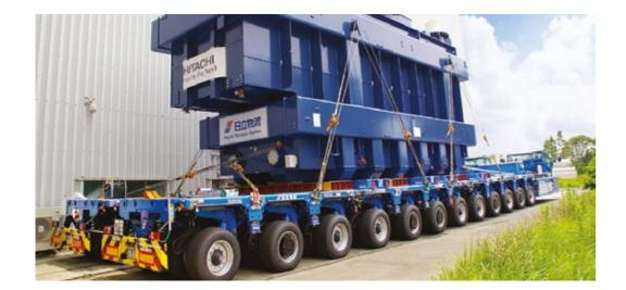
440 t IN JAPAN A parallel combination created with 2x12 axle PST/ES-E moves a generator.
