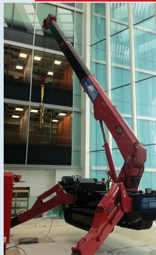
The UNIC 706 is the largest mini crane in the Hird fleet offering a maximum lifting height of 22.7m.
